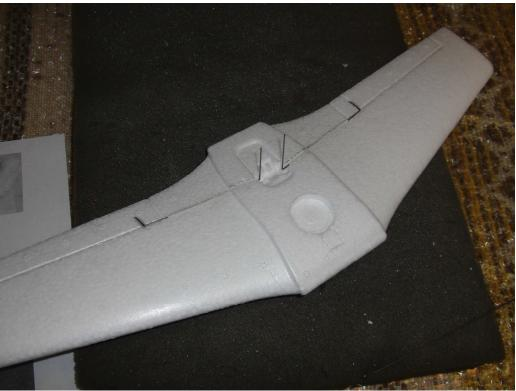
Elevator pushrod installed
