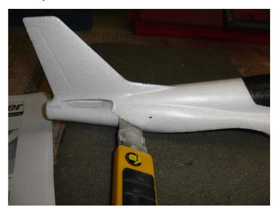
Install torque rod for the elevator and do the same for the ailerons
