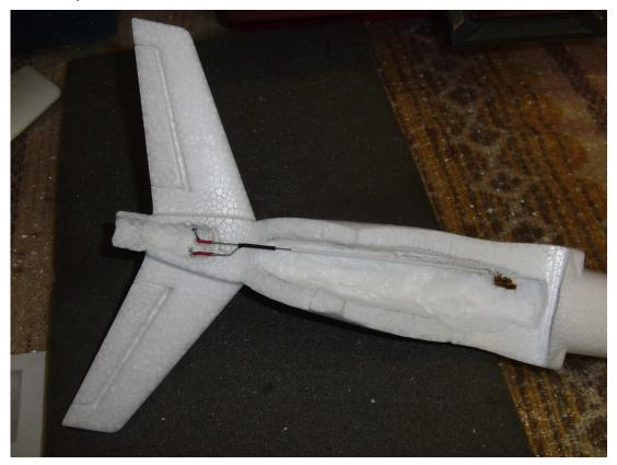
Ailerons servo installed, use 4g servos for control.
